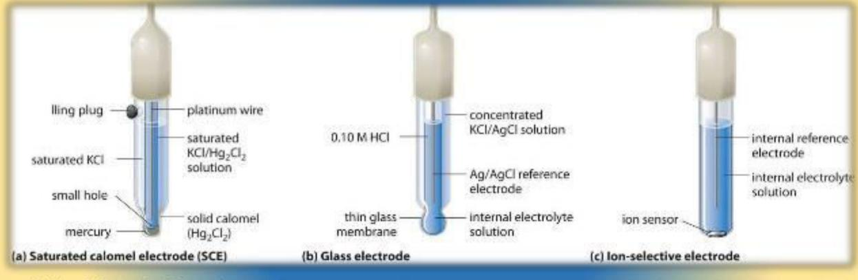
a. Calomel electrode: It consists of a glass tube containing saturated KCL connected to platinum wires through mercury (mercury chloride) b. Glass electrode: It consists thin bulb of special glass blown(lithium) at the end of the glass tube, and the bulb is filled with dilute acid for example decinormal HCL acid connected to a silver chloride electrode
