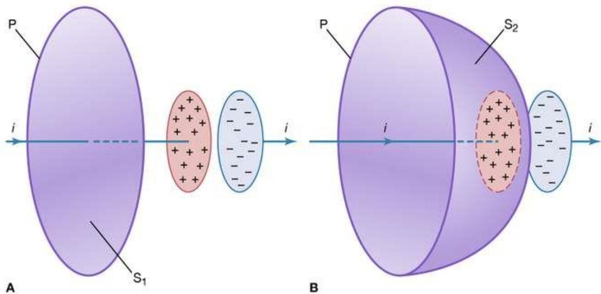
Figure: Current  $i$  charging a capacitor as an illustration of Maxwell's displacement current
