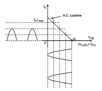
(iii) **Class C power Amplifiers**: If the collector current flows for less than halfcycle of the
