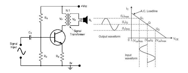
The operating point of this amplifier is present in the linear region. It is so selected that the current flows for the entire ac input cycle. The power amplifier must be biased in such a way that no part of the signal is cut off. As the output wave shape is exactly similar to the input wave shape, therefore such amplifiers have least distortion. They have the disadvantage of low power output and low collector efficiency.
