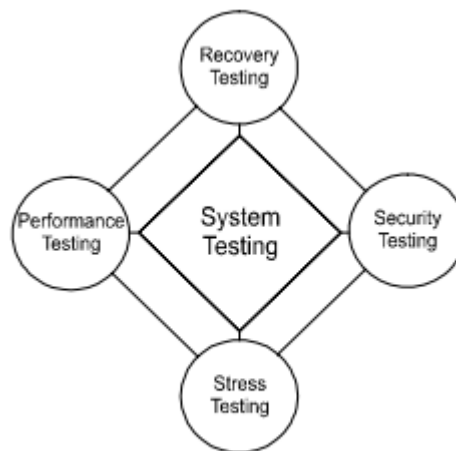
Figure 5.16 Types of System Testing
